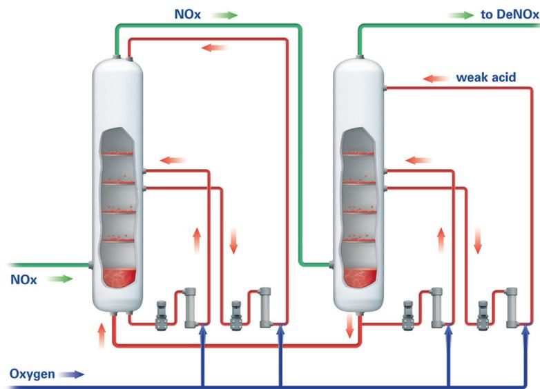
**Figure 3.** Flow chart of the last two absorption towers at NA line 2 with four injection points.
