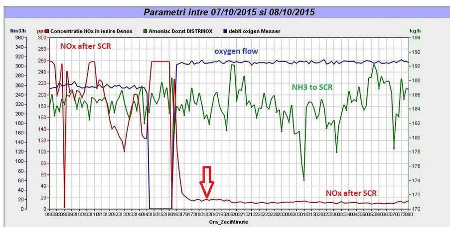
**Figure 6.** Plot of NO<sub>x</sub> values, ammonia consumption and oxygen flow. The red line indicates NO<sub>x</sub> emissions after DeNO<sub>x</sub> (limit value: 90 ppm). The green line indicates NH<sub>3</sub> consumption for DeNO<sub>x</sub>, which was kept at approximately 185 kg/hr. The blue line indicates oxygen consumption, which started at 260 Nm<sup>3</sup>/hr and increased to 310 Nm<sup>3</sup>/hr. NO<sub>x</sub> emission values decreased to 20 ppm.
