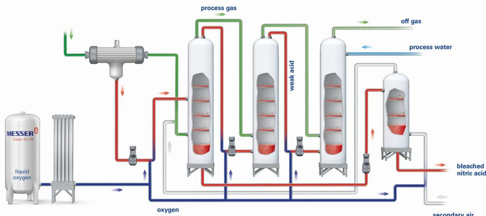
**Figure 1.** Flow chart of nitric acid production with different introduction points.
