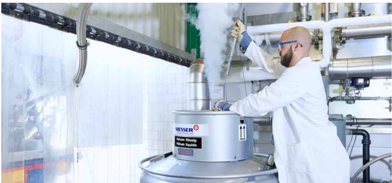
Transfilling of liquid helium in Lenzburg
