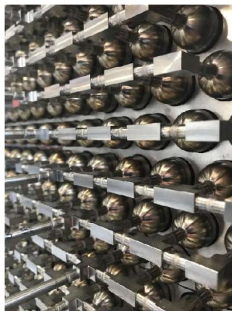
Stacks filled with metal hydride in a compaction unit
